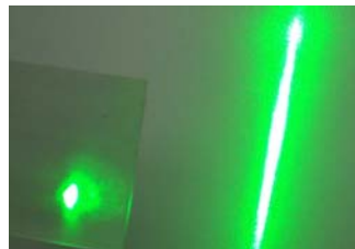
Green Laser going through the TRT sample.
